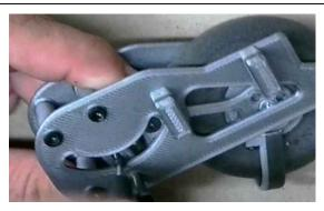
8. Bring the gear in down position and put the drive-lever over the head of the M3 screw, align it to the centre-lever and secure with the M2  $\times$  10mm screw and nut.
