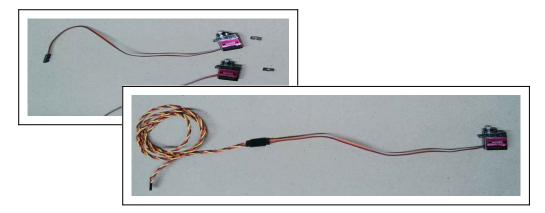
9. Take some 1mm steel wire (>80cm), insert its tip into the extension plug from the back and guide the cable to the wing centre. Now bring the cable and the servo into their pocket and fix the servo with one screw and a spot of silicone or hot glue to the other side of the servo and the wall.
