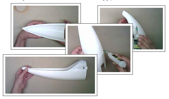
2. Now attach the skins to the main frames. Use a glass plate or mirror and place main frames flat sides onto, then place skin over care for good, even seat before applying glue. Wipe off excess glue and cure. (If stuck to glass slide in snap knife blade from the side to separate.)
