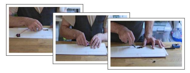
11. Install the pushrod connectors to the third hole of each servo horn.
