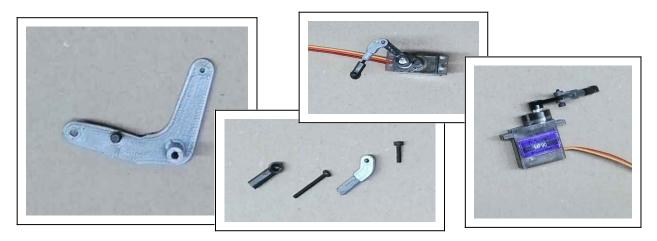
2. Connect left and right lower arm with the M3  $\times$  30mm countersunk screw, press on plane surface, when tightening the screw.
