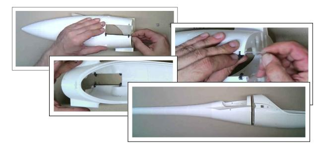
9. Now glue in the four  $\varnothing$  4mm  $\times$  0,5mm brass tubes and sand them flush to the surface.
