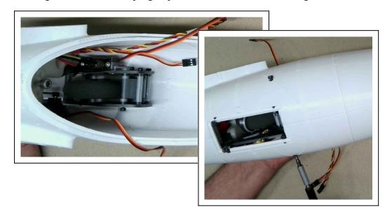
10. Turn over the fuselage and install the gear-doors with the M2 × 8mm countersunk screws, then drive out the gear and hang in a rubber ring into the rear hinges each, turn back the fuse and guide rings to the central locking screw. Check function and adjust rubber tension by including one or both upper M5 screw heads if necessary.
