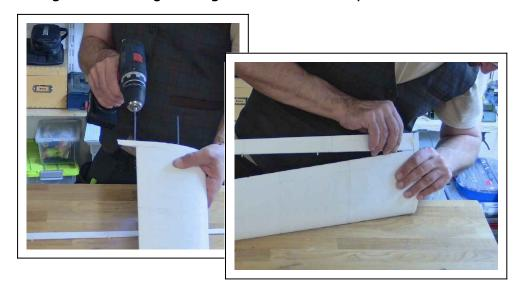
6. If everything is snug, lift flap a bit to bring a <u>tiny</u> amount of glue into the first three closed pockets. Put back in the hinges and care for good alignment to strak and clearance inside the groove, then cure and continue with the last hinge of the opposite site. In this way work through the hinges one by one.
