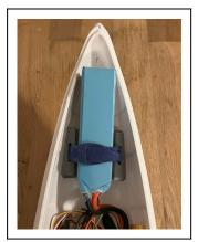
6. Now tidy up the wiring to the final, giving good care to the wheel / EDF area and close the remaining zip ties.
