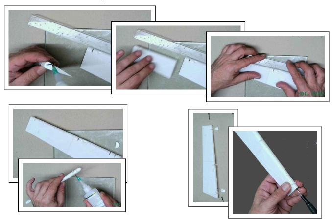
14. Now apply a <u>tiny</u> amount of glue into the opposite pockets in the v-stabilizer and guide hinges in. Aim from top for centred position and sufficient clearance and again check ease of move.
