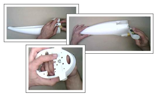
5. Begin with the rear fuselage section by sticking in the three carbon rods to fuselage\_4. Take a look at the cut-outs to assure the long rods reached their final position, then cure.
