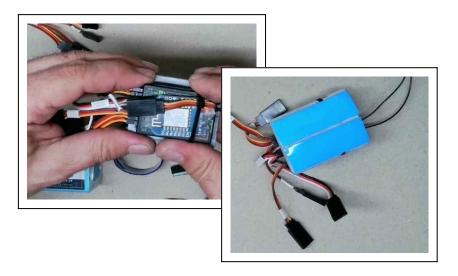
2. Guide the flap and aileron extensions from receiver to the cable openings left and right in the fuselage, arrange and plug in the remaining servo cables to your receiver accordingly and use cable ties and sockets to prepare a clean sweep, but don't tighten the ties completely yet.
