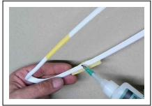
2. Pre assemble the canopy parts, then apply a small line of glue along the joints, wipe off excess glue and allow to evaporate some time before curing to avoid the white glue-shadows. Don't cut away the bars inside yet.
