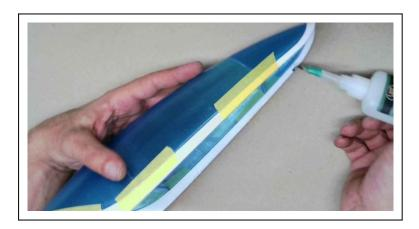
4. Glue a 10mm piece of filament or a Ø 1,8mm × 10mm steel wire (nail) into the hole of the frame as positioning pin and then the hook from inside to the top. Attach a rubber ring to the gear frame, hook the other side to the canopy hook, then guide the pin into the hole in the fuselage and snap on canopy.
