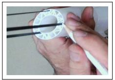
7. Careful apply glue to the face side of the assembly and the marked area on the rods. Avoid the free fuselage-part or other areas of the rods!
