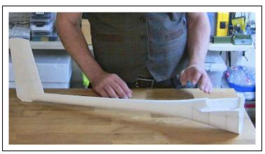
12. (<u>Tip:</u> Use glass plate and a ruler or wood strip as ledge to position the following light-weight parts, like done before with the frame skins.)
