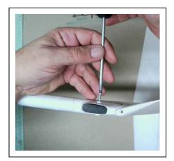
3. Now assemble the wheel levers and install the front wheel with the M3  $\times$  28mm countersunk screws, then attach the wheel guard with two M2  $\times$  10 cylinder screws.
