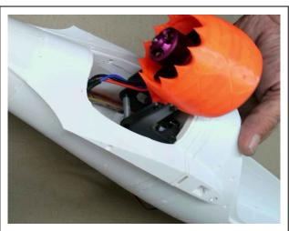
8. Attach the way-extender to the EDF servo, power up and check movement of the unit. Make sure the servo hasn't to work against any resistance in its end positions and adjust the length of the linkage accordingly.
