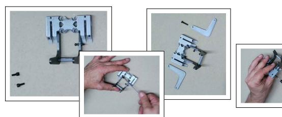
4. Insert EDF unit into its housing, then use  $M2 \times 10$ mm cylinder screws to attach the lower arms and  $M2 \times 16$ mm cylinder screws for the upper arms. Now use a snap knife and adopt your EDF inlet funnel to the cut outs for the upper arms. Make sure the arms can operate easily and undistracted and tighten screws carefully. Use a drop of CA to the thread if the screw is too loose.
