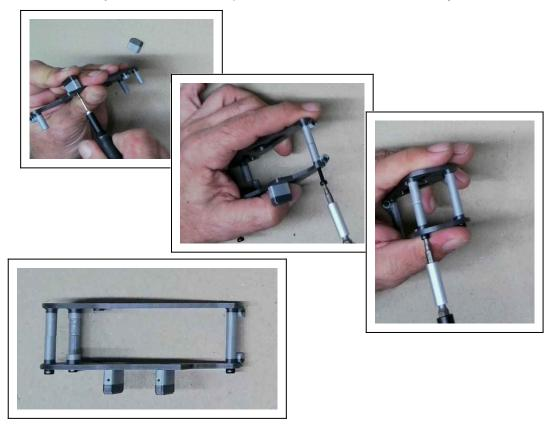
6. Link the centre-lever with the drive-shaft from the left and the M3  $\times$  12mm from right, then lock with the M3  $\times$  18mm screws, but be careful, don't overdo! Now check torque transmission with an Allen key.
