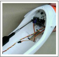
7. Connect the ESC extension cables to the fan motor, guide them in an arc, giving enough way to allow undistracted movement of the EDF unit and unite them with the rudder- and elevator servo cable. Now guide the bunch through the hole in the left side of the main-frame and secure carefully inside the engine bay with a strip of duct tape.
